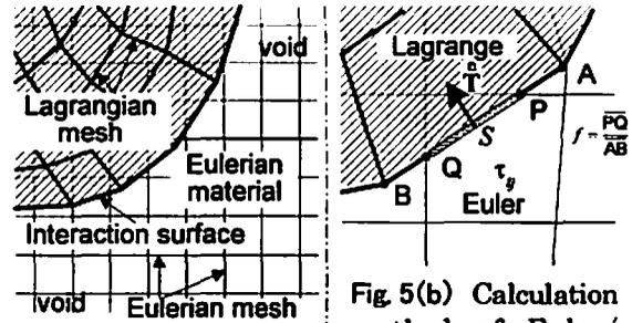
Fig 5(a) Schematics depicting the Euler/Lagrange interaction.
