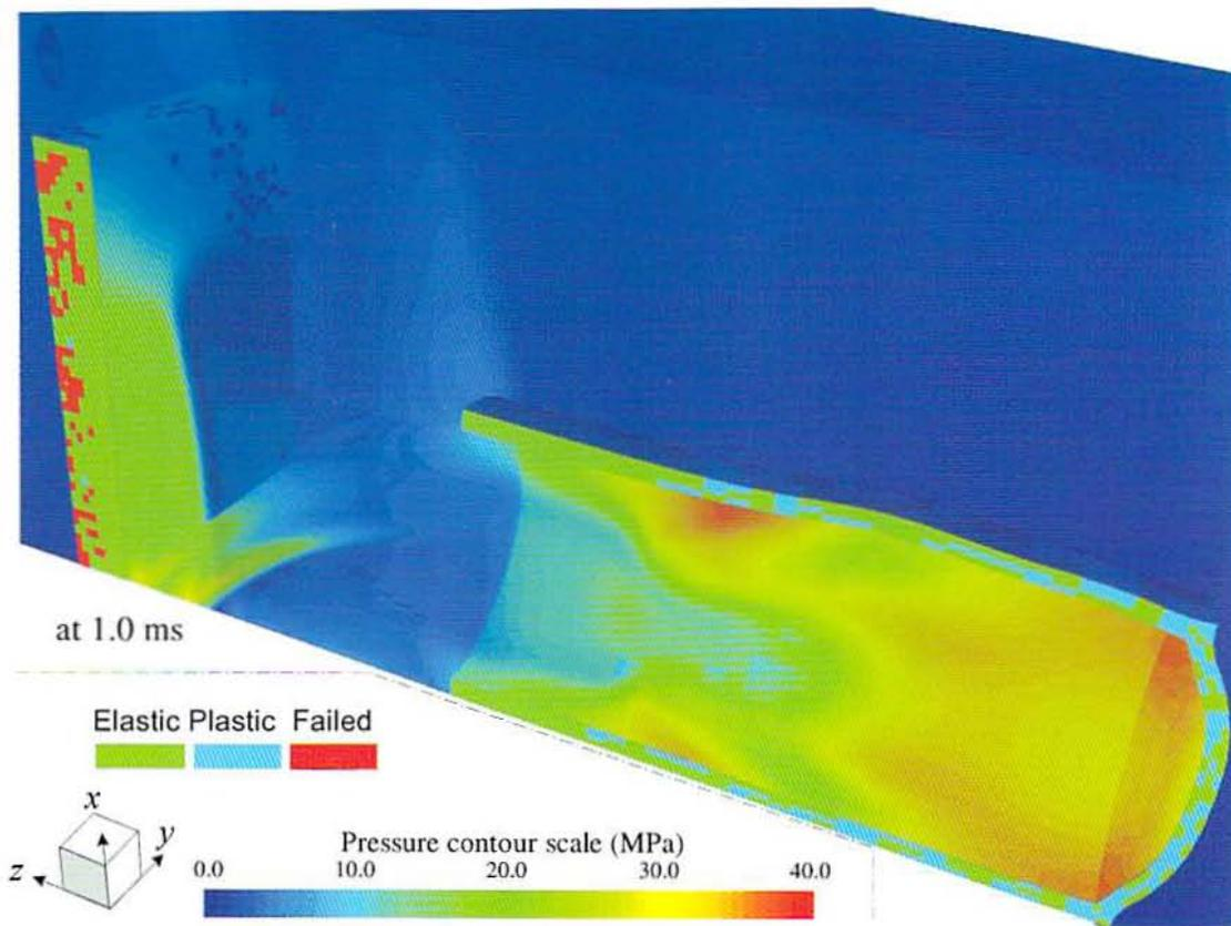
Fig. 8 Transparent pressure contour in the fluid and material status map in the structures.
