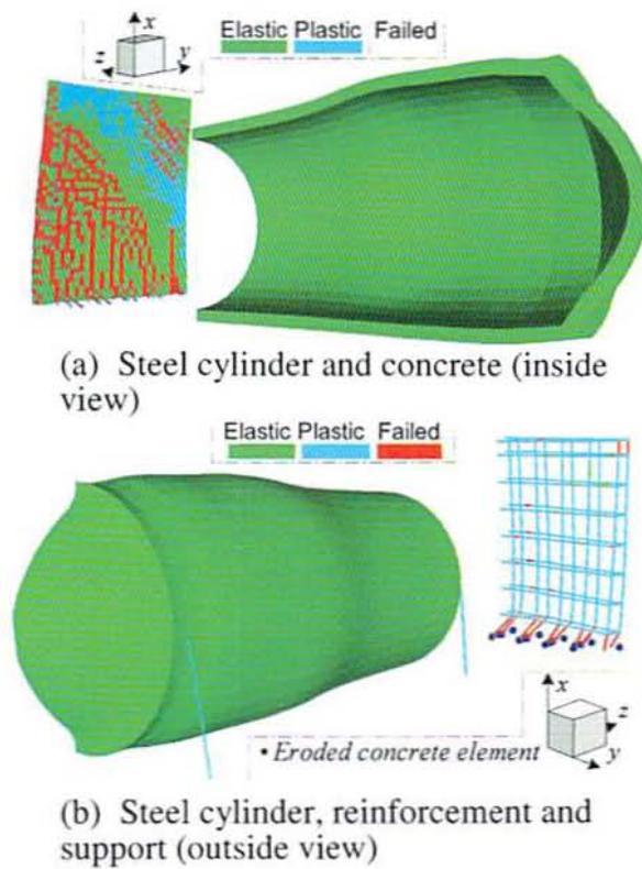
Fig. 10 Material status map in the structures at 5.0 ms.
