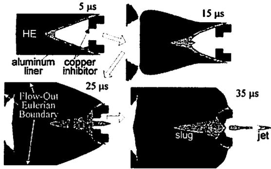
Fig. 6 Trapping process of the slug by the inhibitor simulated numerically.
