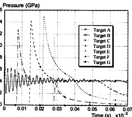
Fig. 11 Pressure histories in the TNT during one-dimensional preliminary analysis.
