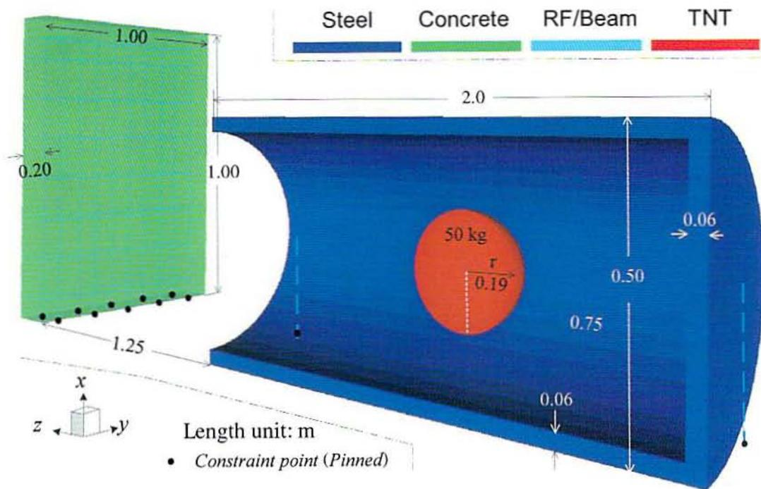
Fig. 7 Numerical analysis model and its geometrical dimensions.
