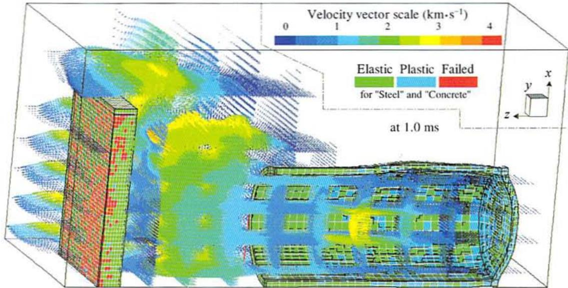
Fig. 9 Velocity vector distribution in the fluid and material status map in the structures.
