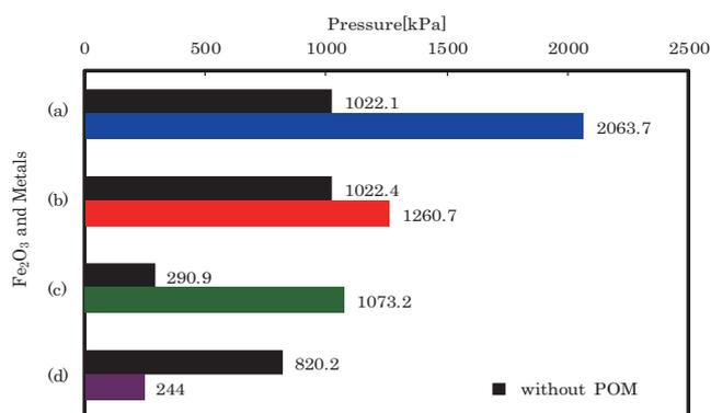
**Figure 7** Comparison of the maximum pressure obtained from Fe<sub>2</sub>O<sub>3</sub>/metal and Fe<sub>2</sub>O<sub>3</sub>/metal/POM (5/5/20) mixtures, following (a) Fe<sub>2</sub>O<sub>3</sub>/Al, (b) Fe<sub>2</sub>O<sub>3</sub>/Mg, (c) Fe<sub>2</sub>O<sub>3</sub>/Ti and (d) Fe<sub>2</sub>O<sub>3</sub>/MgAl.
