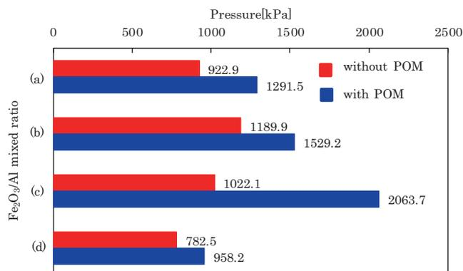
**Figure 5** Comparison of the maximum pressures obtained from Fe<sub>2</sub>O<sub>3</sub>/Al and Fe<sub>2</sub>O<sub>3</sub>/Al/POM mixtures, following (a) 7/3, (b) 6/4, (c) 5/5 and (d) 4/6.
