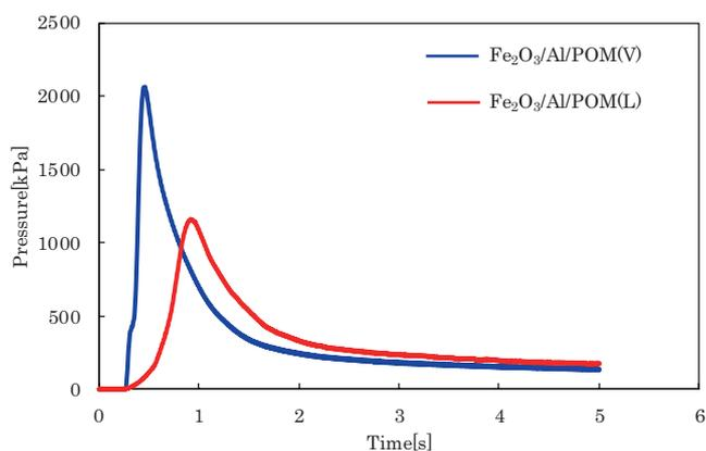
**Figure 4** Combustion test results for Fe<sub>2</sub>O<sub>3</sub>/Al/POM mixtures formulated with vigorous (V) and light (L) mixing.
