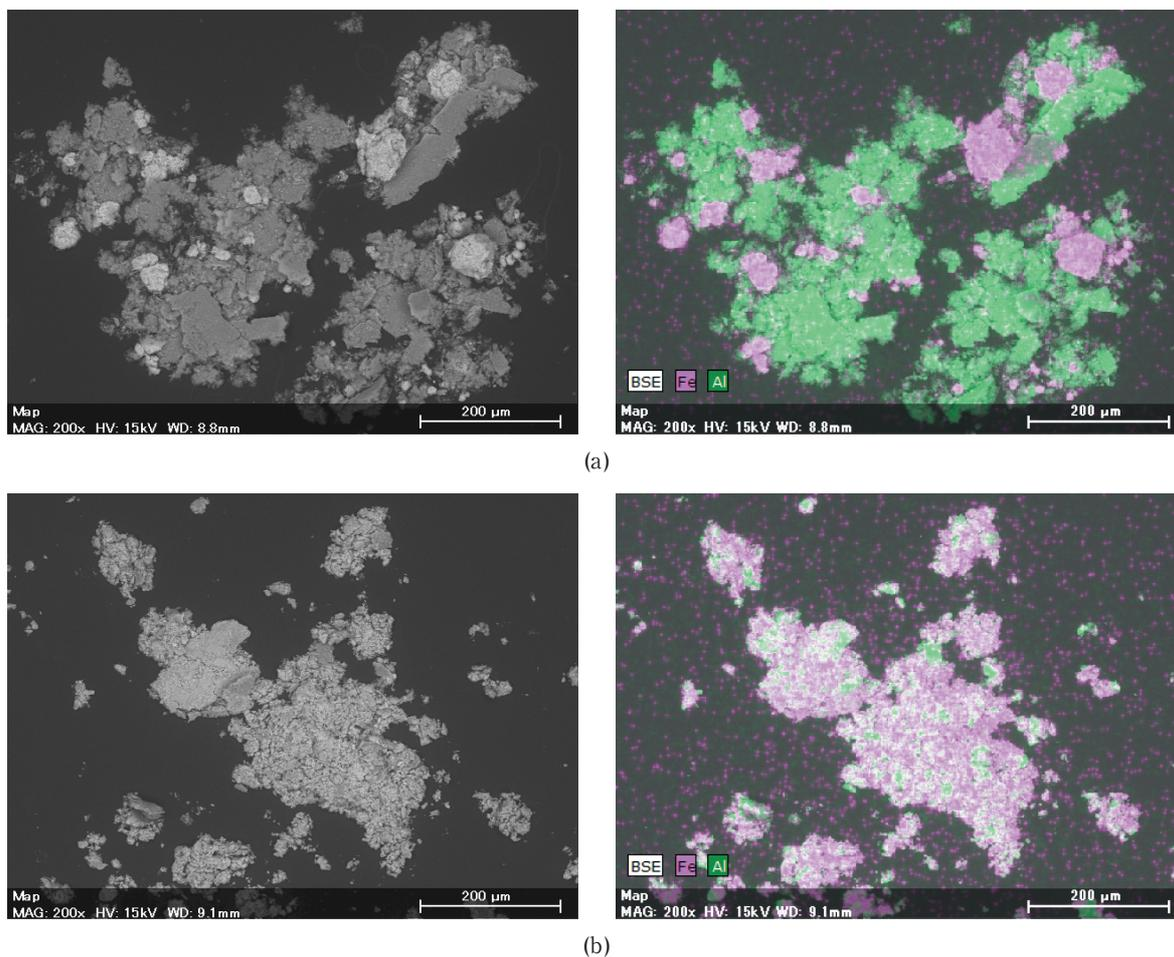
**Figure 2** SEM and EDS images of  $\text{Fe}_2\text{O}_3/\text{Al}$  mixture used in this study, following (a) light and (b) vigorous mixing.
