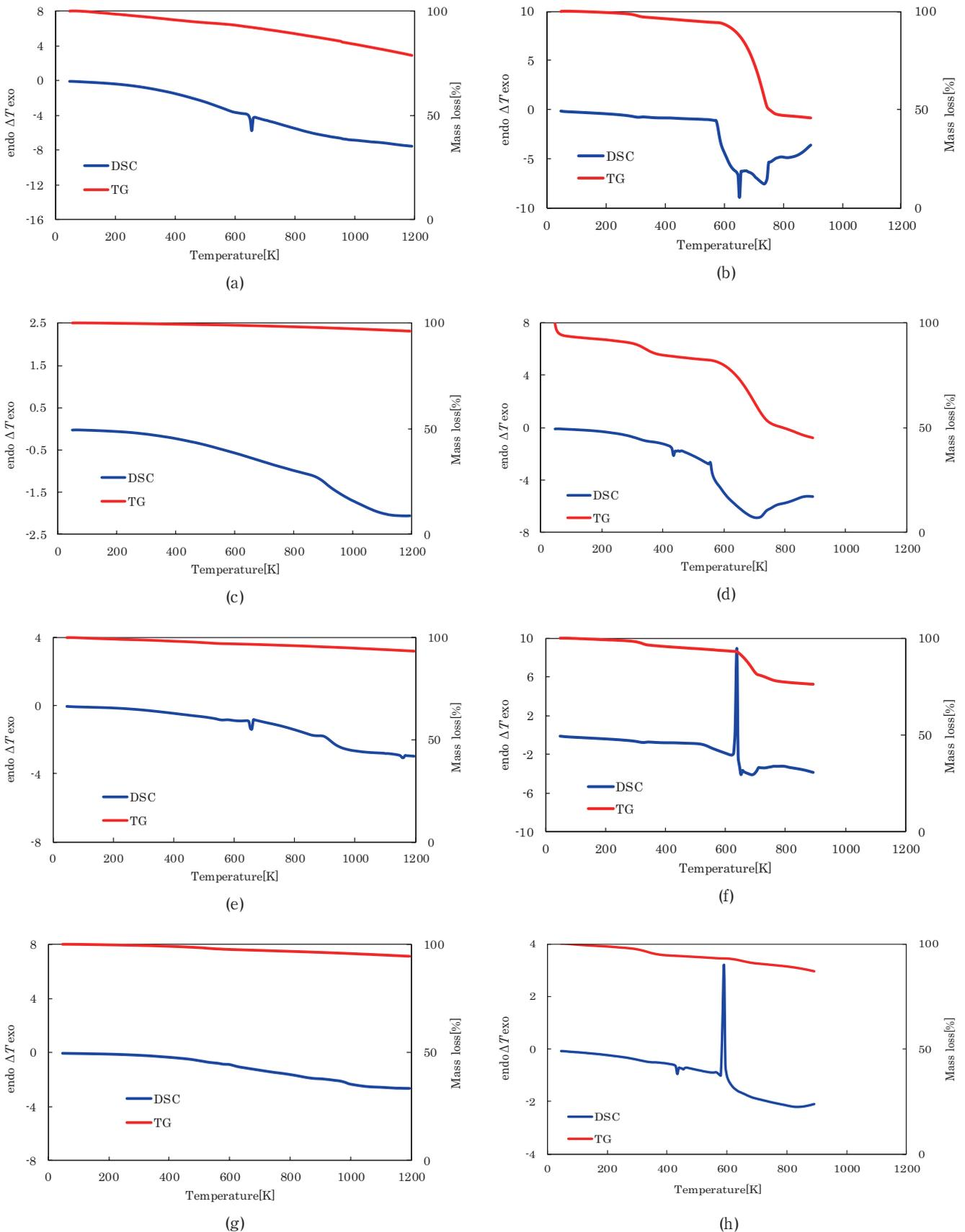
**Figure 3** TG-DSC curves obtained for (a) Al, (b) Mg, (c) Ti, (d) MgAl and 1 : 1 (e) Fe<sub>2</sub>O<sub>3</sub>/Al, (f) Fe<sub>2</sub>O<sub>3</sub>/Mg, (g) Fe<sub>2</sub>O<sub>3</sub>/Ti and (h) Fe<sub>2</sub>O<sub>3</sub>/MgAl mixtures.
