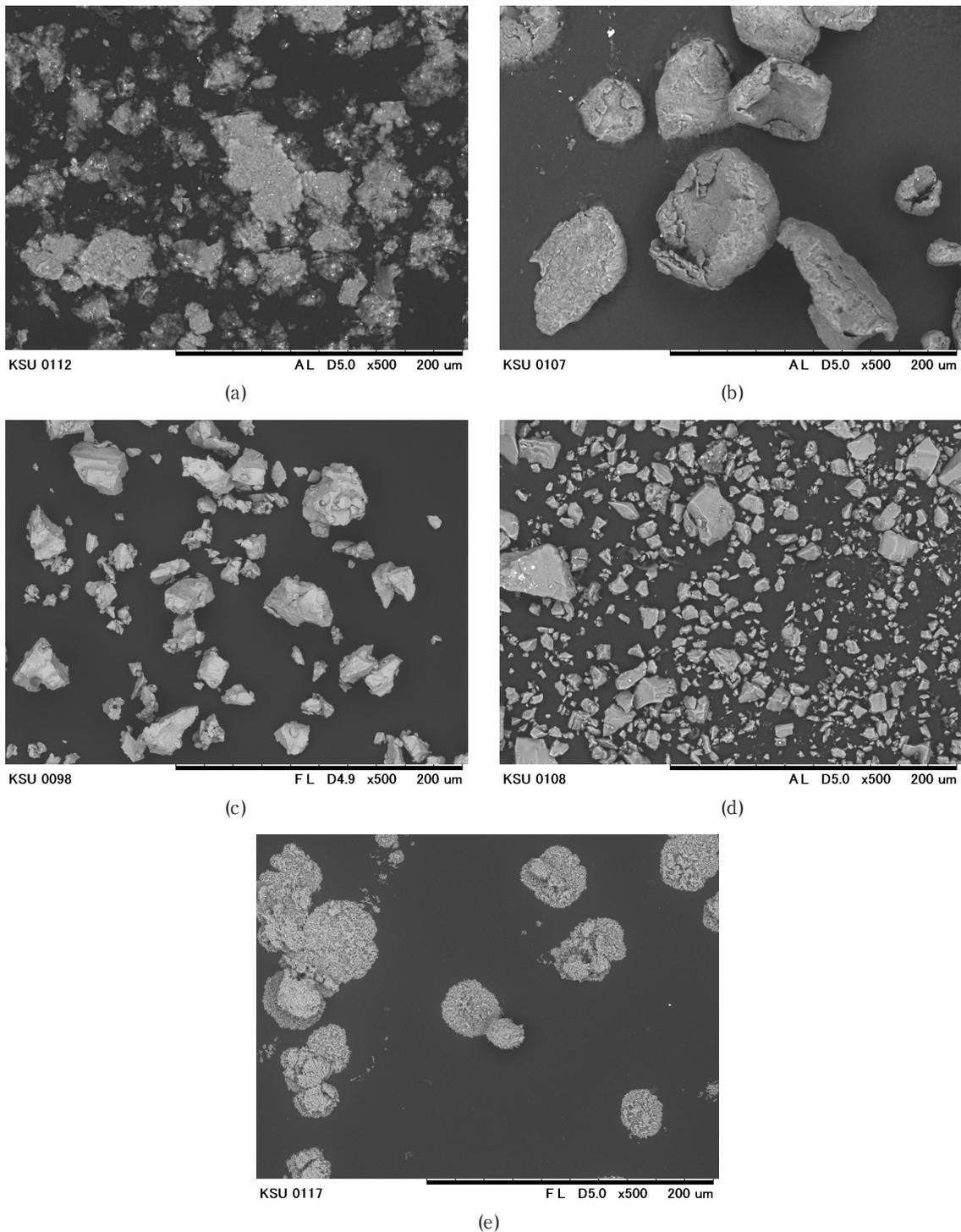
Figure 1 SEM images of (a) Al, (b) Mg, (c) Ti, (d) MgAl and (e) Fe<sub>2</sub>O<sub>3</sub> used in this study.
