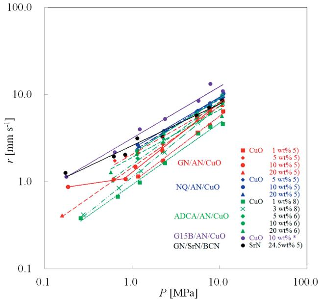
**Figure 2** Linear burning rate data for AN based mixtures and GN/SrN/BCN mixture. (\*denotes the set of data that were acquired in this study.)
