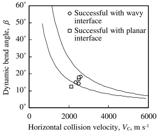
Fig. 6 Weldability window for Ti / SUS 304 clads (3 mm flyer thickness).
