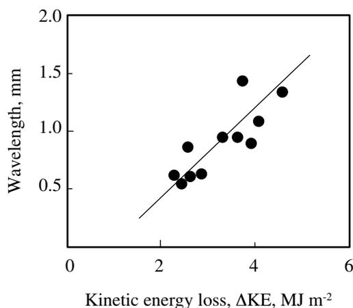
Fig. 4 Variation of wavelength with kinetic energy loss,  $\Delta KE$ .
