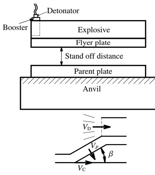
Fig. 1 Schematic of parallel plate configuration of explosive welding and the parameters.
