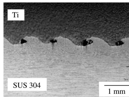
Fig. 2 Optical micrograph of welded interface showing maximum reacted vortex layer.
