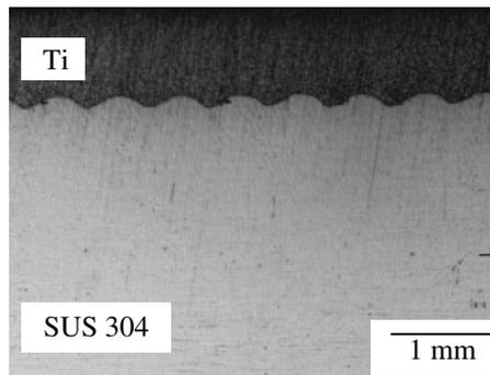
Fig. 3 Optical micrograph of welded interface with less reacted vortex layer.
