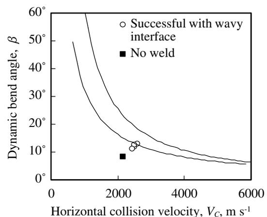
Fig. 5 Weldability window for Ti / SUS 304 clads (5 mm flyer thickness).
