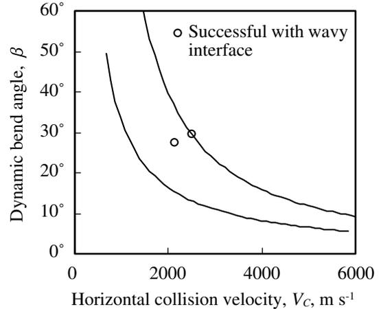
Fig. 7 Weldability window for Ti / SUS 304 clads (1 mm flyer thickness).
