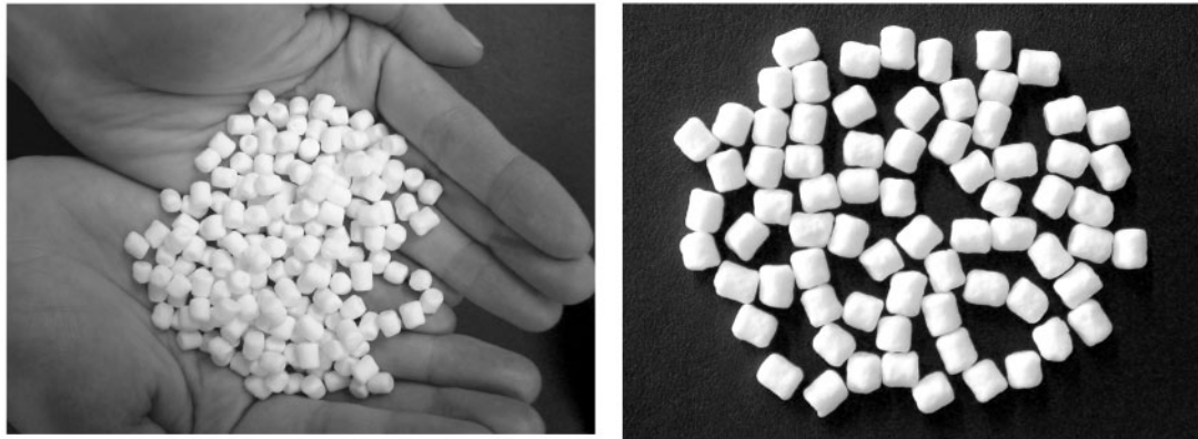
Fig. 1 Granular emulsion explosives (Diameter: 4 mm, Length: 4 mm).
