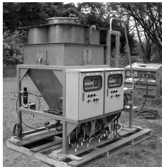
Fig. 5 Loading machine of granular emulsion explosives.
