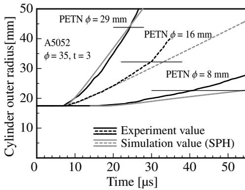
Fig. 8 Numerical and experimental wall radii for smooth cylinders.
