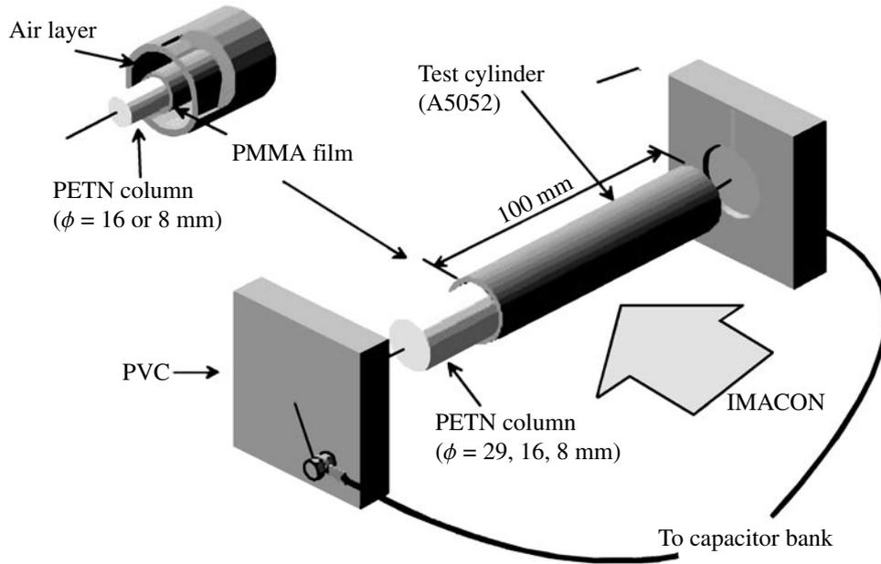
Fig. 1 Schematics of explosion test cylinder.
