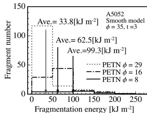
Fig. 10 The comparison of fragmentation energy in each the diameter of PETN column.
