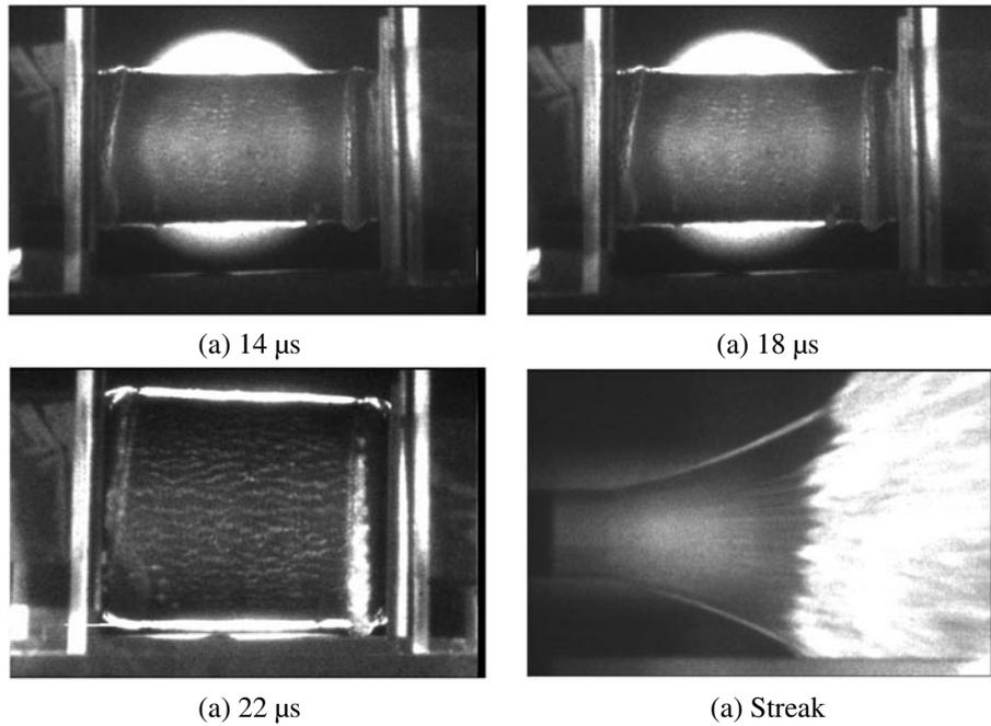
Fig. 5 Framing record of explosion A5052 cylinder for IMACON. ( $\phi_{out}=35$  mm,  $t=3$  mm, PETN  $\phi=29$  mm)
