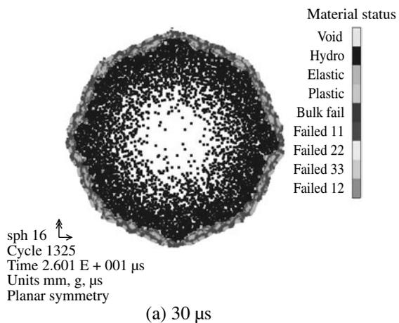
Fig. 7 Numerically expanding and fragmenting smooth cylinder (PETN  $\phi=16$  mm).
