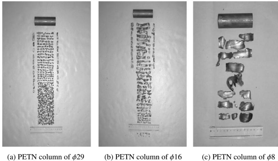
Fig. 3 A photograph of recovery fragments of A5052 cylinder.
