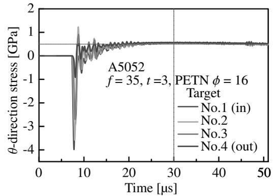
Fig. 9 Numerical time-history of circumferential stresses in the wall of smooth cylinder. (PETN φ =16 mm)
