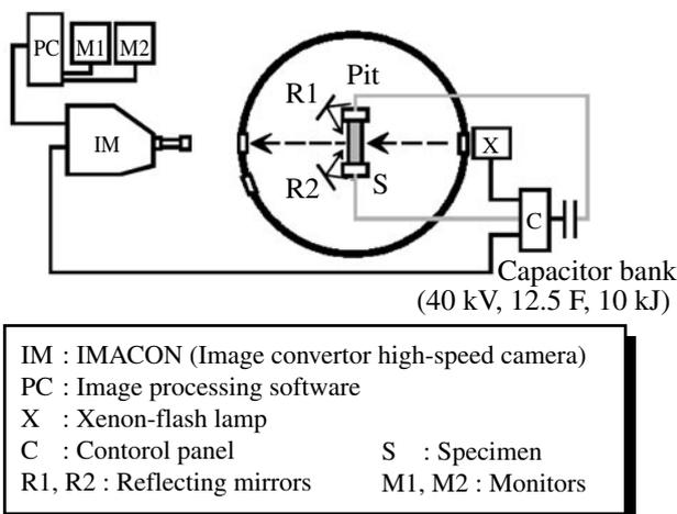
Fig. 4 Schematics of photography test by IMACON.
