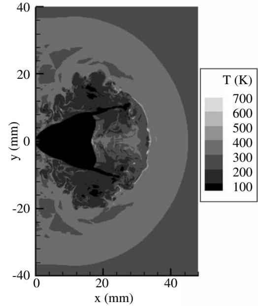
Fig. 9 Temperature contours at 70  $\mu$ s of 70 MPa case.
