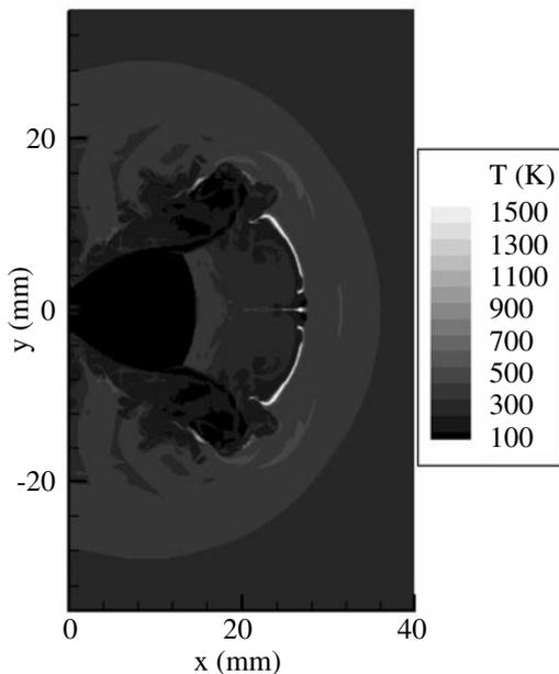
Fig. 10 Temperature contours at 50  $\mu$ s using 10  $\mu$ m grid size of 70 MPa case.
