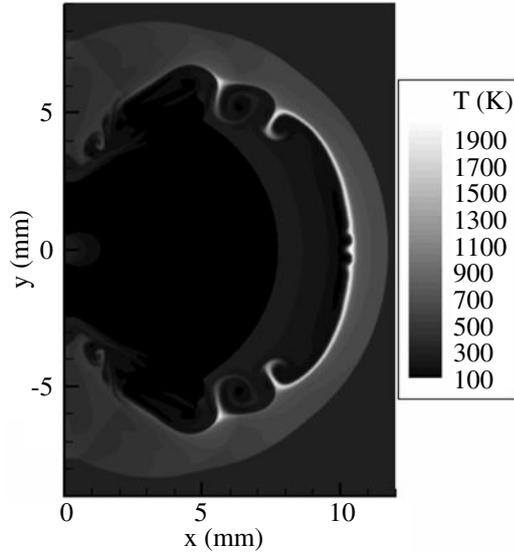
Fig. 8 Temperature contours at 9  $\mu$ s of 70 MPa case.
