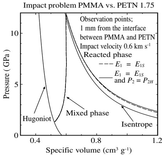
Fig. 5 Loci of the reacted component on  $P$ - $V$  plane during the shock initiation process with the Hugoniot line for reacted component.
