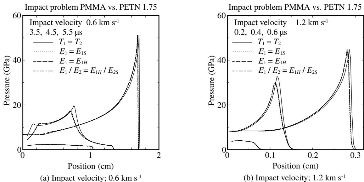
Fig. 1 Numerical results of shock to detonation transition (SDT) process in PETN. The position is counted from the initial interface between the PMMA and PETN.
