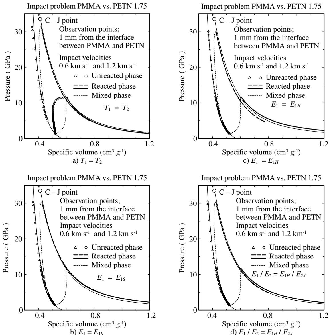
Fig. 4 Loci of the unreacted and the reacted components on  $P$ - $V$  plane during shock initiation process, the state quantities are extracted from the numerical simulation of shock initiation process, impact problems PMMA vs. PETN.
