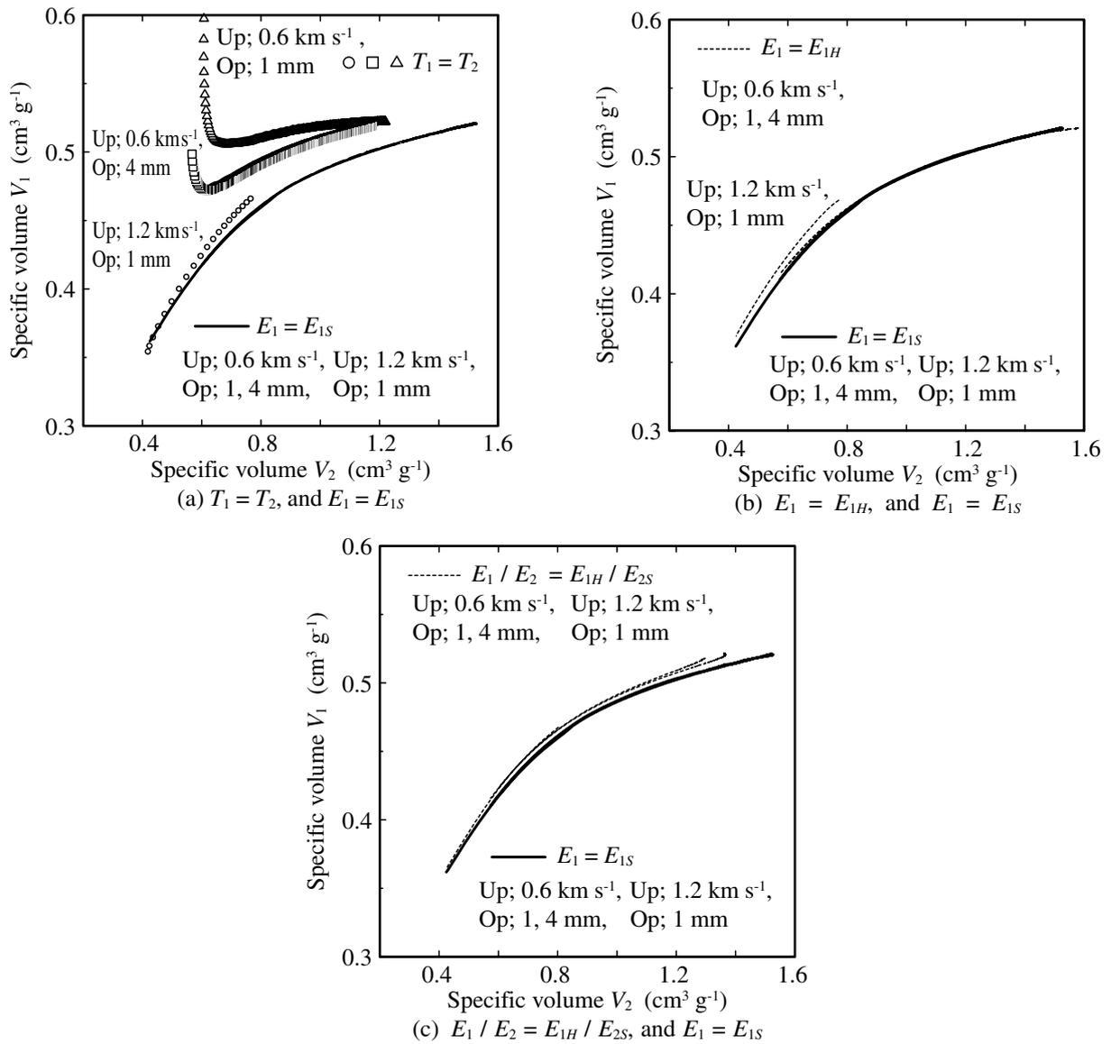
Fig. 2 Relation of the specific volumes of the unreacted and the reacted component in reaction zone of PETN, the state quantities are extracted from the numerical simulation of shock initiation process, impact problems PMMA vs. PETN. Up; impact velocity, Op; Distance from interface of PMMA and PETN to the observation point.
