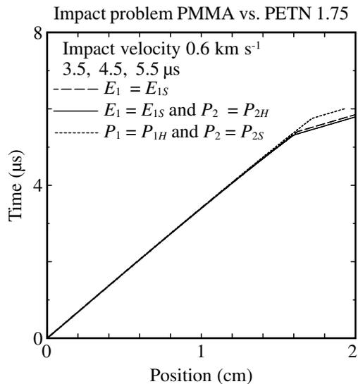
Fig. 7 The x-t diagram on shock propagation process in PETN.
