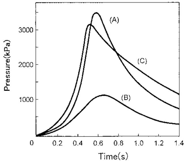
**Fig. 4** Time history of pressure for the mixtures of composition A with poly (oxymethylene) and black powder.
