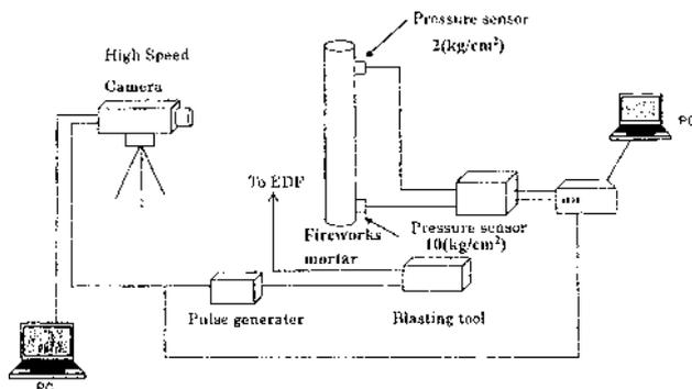
Fig. 2 Experimental setup for the measurement of pressure inside the firework mortar, and exit velocity of aerial shells by framing camera.
