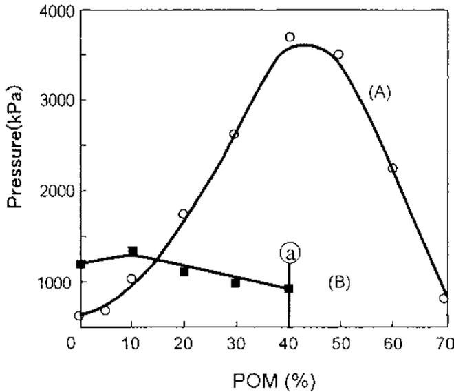
**Fig. 3** Relation between poly (oxymethylene) content (%) and maximum pressure.
