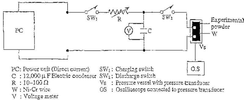
Fig. 1 Pulse discharge circuit for time pressure measurement.
