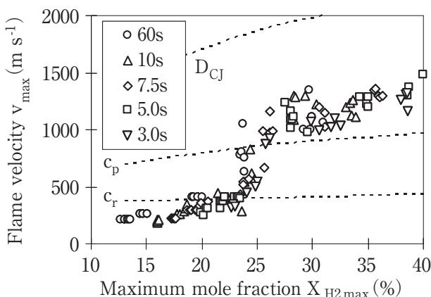
**Fig.5** Maximum flame velocity in the unobstructed part of the tube vs. maximum hydrogen mole fraction.
