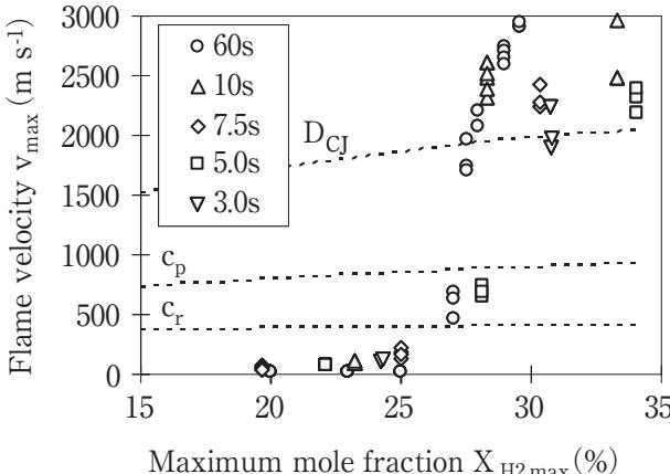
**Fig. 3** Flame velocity vs. maximum hydrogen mole fraction for different vertical concentration gradients.
