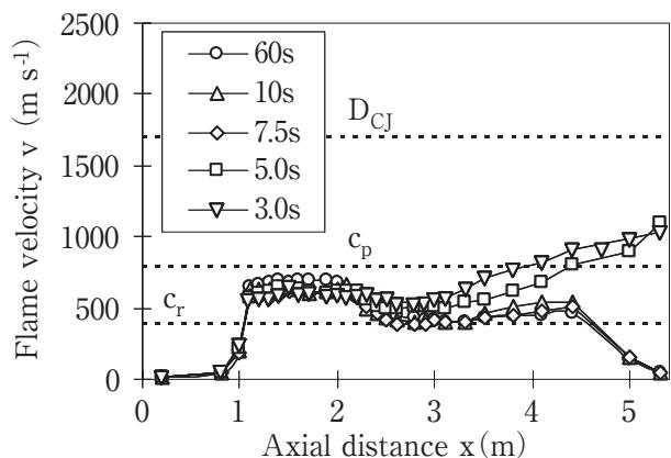
**Fig. 4** Flame velocity vs. axial tube distance with 20 vol.-% hydrogen (global). The obstacle configuration in the tube is :  $BR = 60\%$  and  $S = 100$  mm. The final obstacle is located at 2.05 m.
