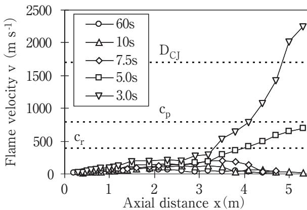
**Fig. 2** Flame velocity vs. axial tube distance for different vertical concentration gradients (waiting time). All mixtures have a global hydrogen content of 20 vol.-%.
