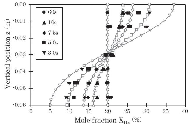
**Fig. 1** Fuel concentration over channel height for different waiting times. The mixture is globally lean with an overall mole fraction of 20 vol.-% fuel. Solid symbols indicate experimental results, transparent symbols numerical results.
