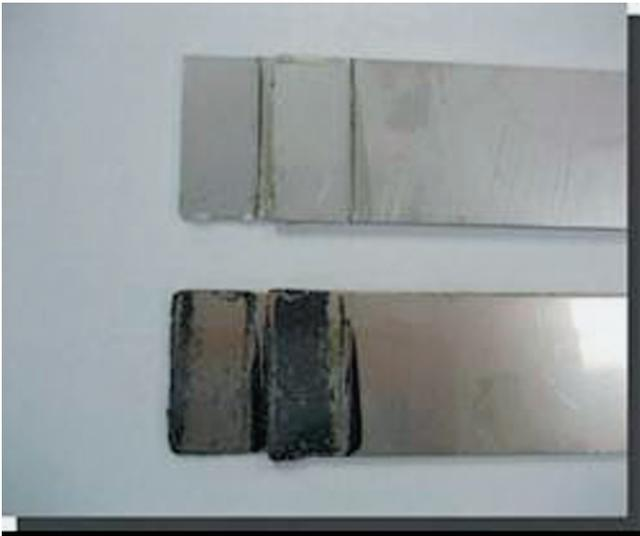
Figure 2 Adhesive interface states before and after heating.
