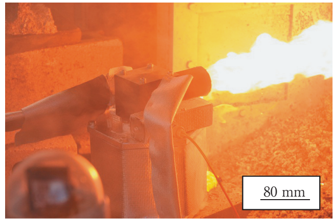
Figure 9 Lithium gas ejection during the ground test.
