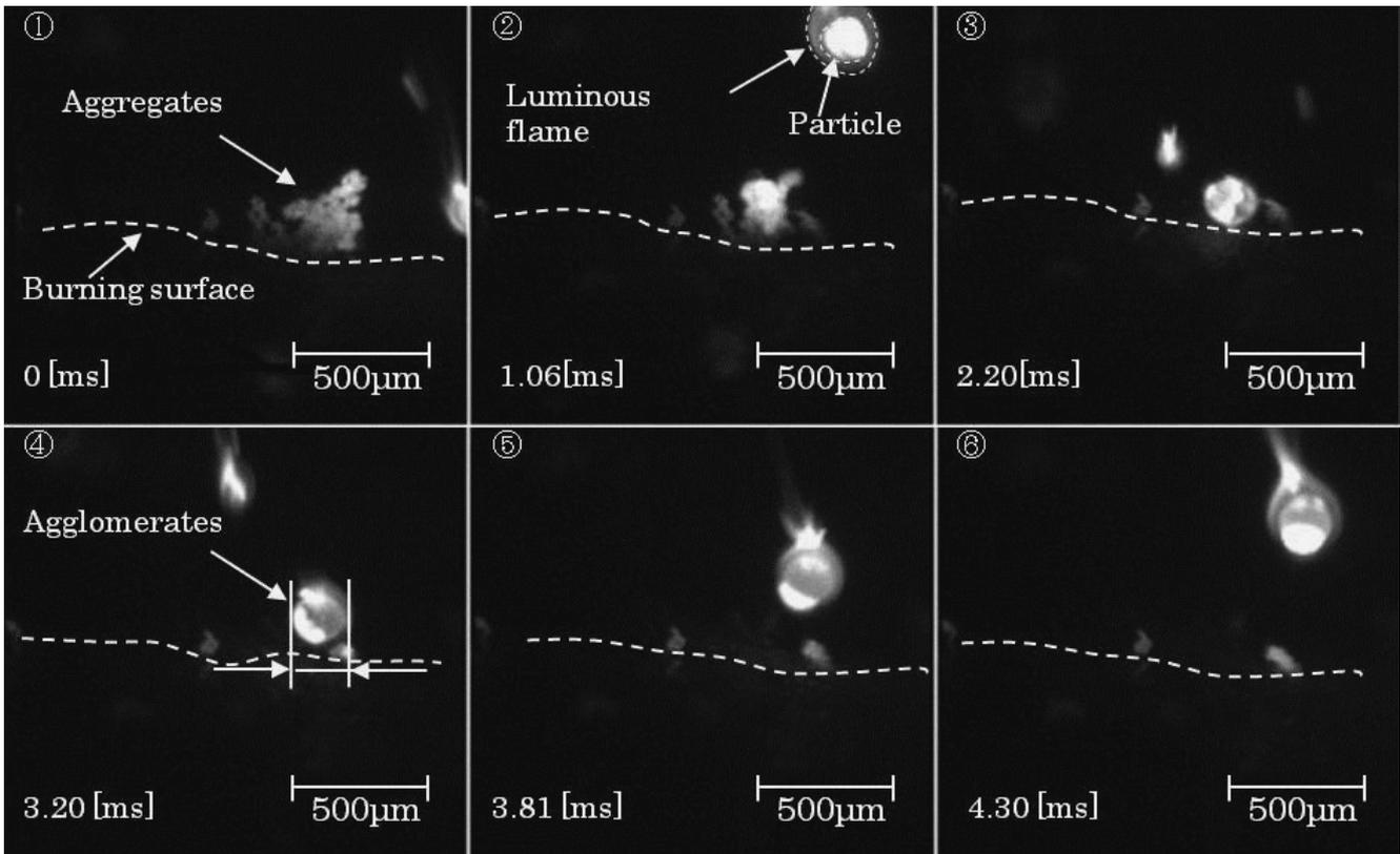
Figure 4 Agglomerate formation at burning surface (AN10–Al20 parts).
