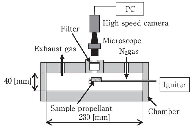
Figure 3 Experimental apparatus of burning surface observation.
