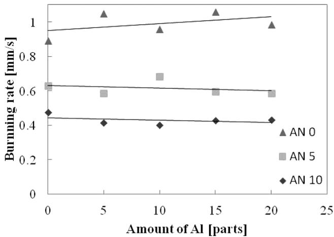
Figure 2 Burning rate for each composition.
