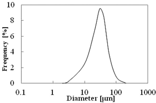
Figure 1 Particle size distribution of Al.
