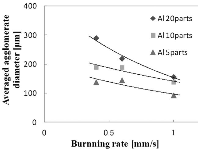
Figure 5 The relation of burning rate and averaged agglomerate diameter.
