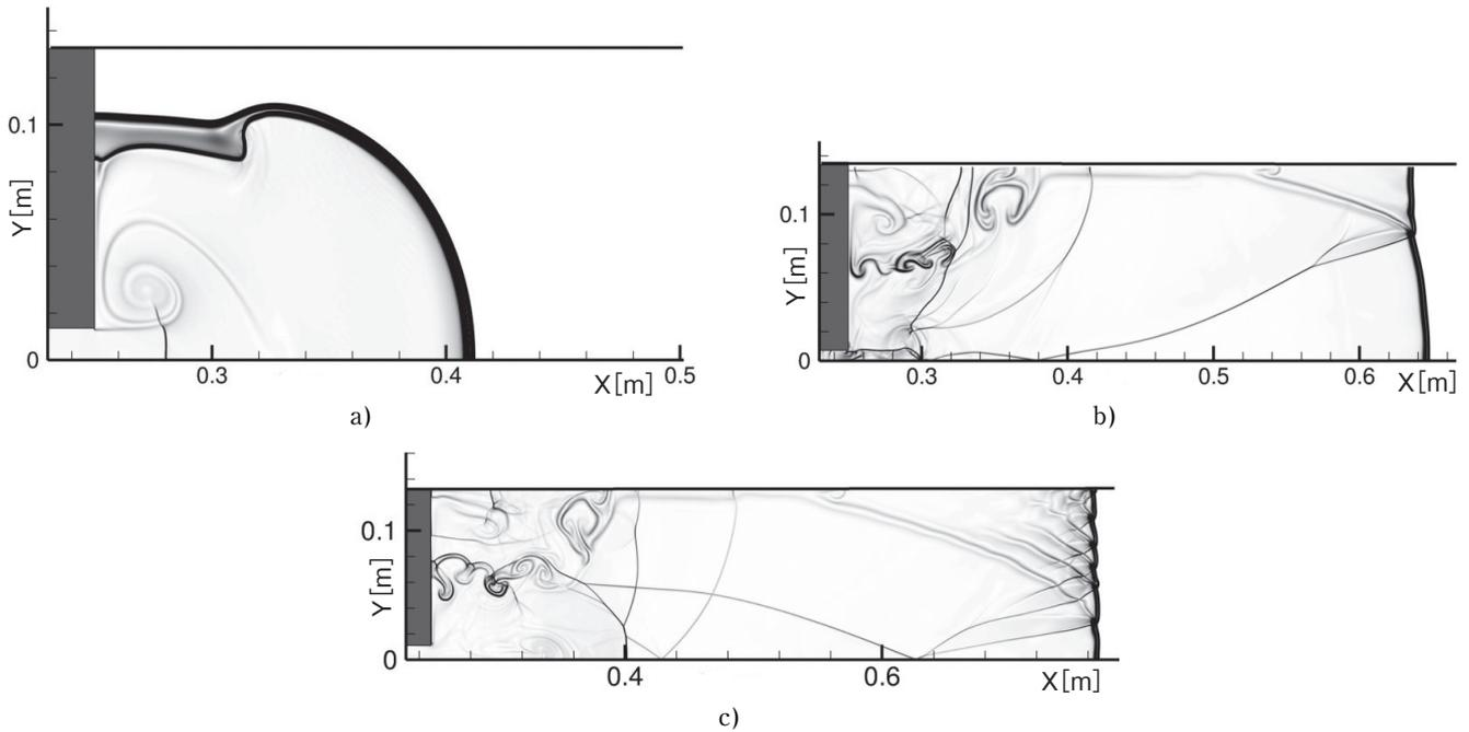
**Figure 3** Critical regime with primary reflection of the detonation part of the diffracted front ( $d = 2\mu\text{m}$ ,  $H_1 = 0.013\text{m}$ ,  $H_2 = 0.132\text{m}$ ):  $t = 0.24$  ms (a),  $0.4$  ms (b),  $0.48$  ms (c).
