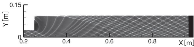
**Figure 6** Maximal pressure histories of cellular detonation transition:  $d = 1.5\mu\text{m}$ ,  $H_1 = 0.033\text{m}$ ,  $H_2 = 0.1\text{m}$ .
