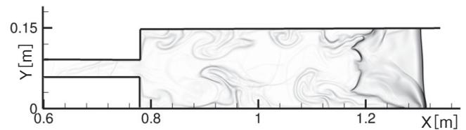
**Figure 8** Detonation failing:  $d = 3.5\mu\text{m}$ ,  $2H_1 = 0.033\text{m}$ ,  $2H_2 = 0.15\text{m}$ ,  $t = 0.75\text{ms}$ .
