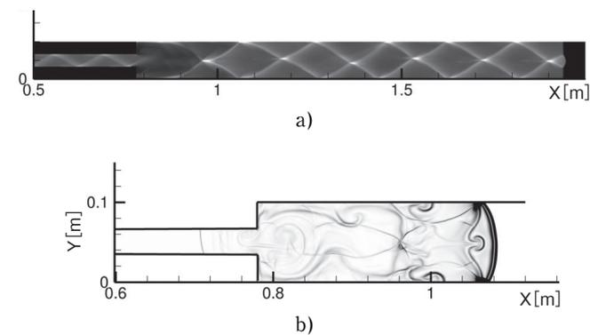
**Figure 7** Reestablishment of cellular detonation in a subcritical regime,  $d = 3.5\mu\text{m}$ ,  $2H_1 = 0.033\text{m}$ ,  $2H_2 = 0.1\text{m}$ : maximal pressure history (a); numerical Schlieren,  $t = 0.25\text{ms}$  (b).
