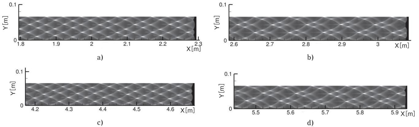
**Figure 5** Transformations of the cellular structures during detonation propagation in wide part of the channel ( $d = 2\mu\text{m}$ ,  $H_1 = 0.012\text{m}$ ,  $H_2 = 0.066\text{m}$ ):  $K \sim 30$  (a), 40 (b), 60 (c), 80 (d).
