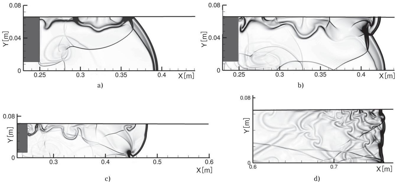
**Figure 4** Detonation restoration in a subcritical regime ( $d = 2\mu\text{m}$ ,  $H_1 = 0.011\text{m}$ ,  $H_2 = 0.066\text{m}$ ):  $t = 0.24$  ms (a),  $0.28$  ms (b),  $0.32$  ms (c),  $0.5$  ms (d).
