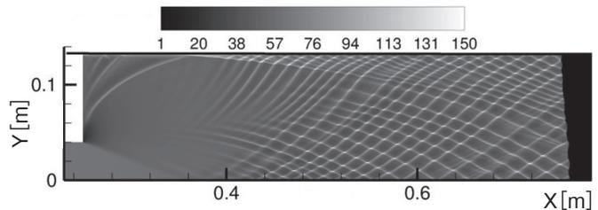
Figure 2 Initial stage of the cellular detonation formation in the supercritical regime,  $d = 1\mu\text{m}$ ,  $H_1 = 0.04\text{m}$ ,  $H_2 = 0.132\text{m}$  (maximal pressure histories).
